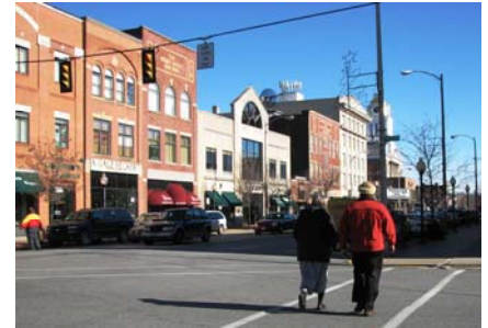
Figure 5.1: Pedestrian facilities such as this crosswalk in Indiana Borough allow people to travel easily and safely on foot. This intersection employs striped pavement for the crosswalk as well as crossing signs with audible signals.
